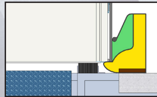
Dual Compression & Wiper Seal for Standard Trailers
