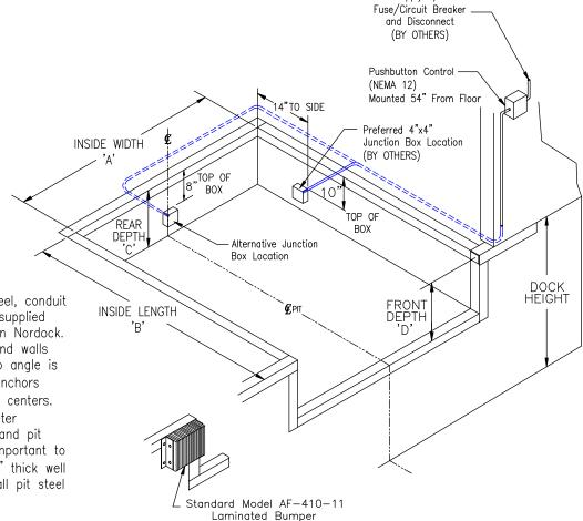
All pit construction, pit steel, conduit and bumper anchors are supplied and installed by other than Nordock. Keep all corners square and walls plumb. Recommended curb angle is 3" x 3" x 1/4" with 6" anchors attached on minimum 12" centers. Conduit to be 3/4" diameter terminated at power unit and pit location as shown. It is important to maintain a minimum of 8" thick well vibrated concrete behind all pit steel and down dock face.
