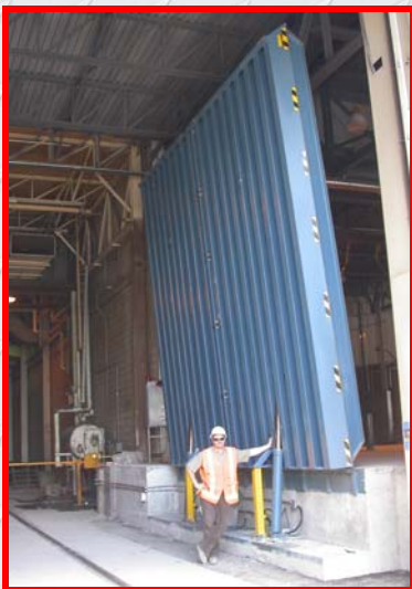
20' X 20' 30,000 POUND CAPACITY DUAL LANE RAIL BRIDGE
