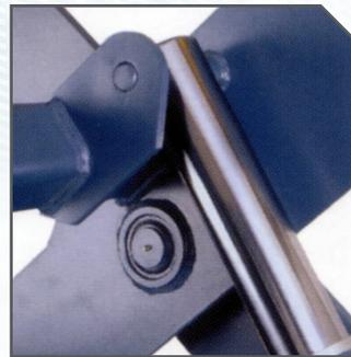
Self-Aligning spherical bearings at center of scissors and cylinder base alleviate stress, improve efficiency and extends product life.
