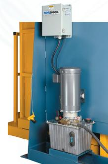
Power unit with 3 Phase TEFC motor, gear pump, valve manifold, filters and oil filled reservoir.
