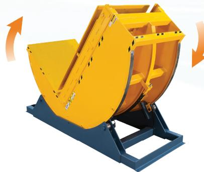
**STEP 2** | Once secured, the operator safely inverts the load a full 90° at the push of a button.
