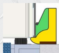
Dual Compression & Wiper Seal For Standard Trailers
