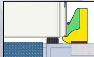
Dual Compression & Wiper Seal for Standard Trailers
