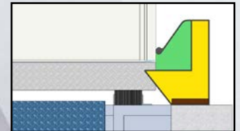
Wiper Seal for Trucks Equipped With Step or Tailgate
