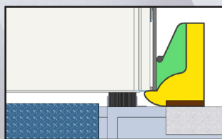
Dual Compression & Wiper Seal for Standard Trailers
