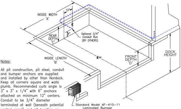
and installed by other than Nordock. Keep all corners square and walls plumb. Recommended curb angle is  $3" \times 3" \times 1/4"$  with 6" anchors attached on minimum 12" centers. Conduit to be 3/4" diameter terminated at wall (beneath potential control panel) and pit location as shown. It is important to maintain a minimum of 8" thick well vibrated concrete behind all pit steel and down dock face.
