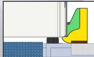
Dual Compression & Wiper Seal for Standard Trailers
